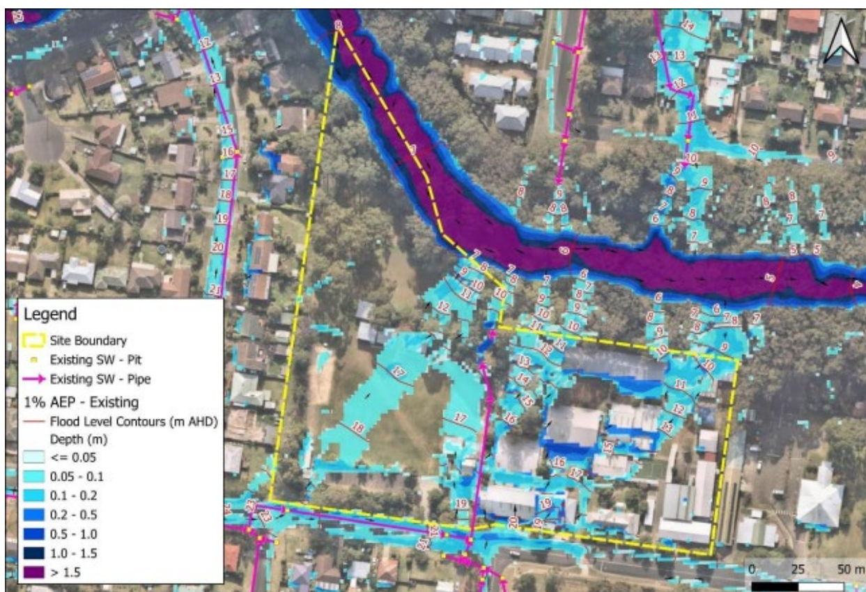
Figure 23 Existing scenario - peak flood levels and depths at the site in the 1% AEP
