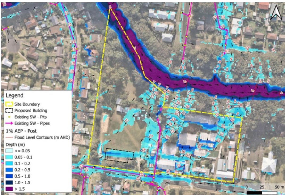
Figure 25 Proposed scenario - peak flood levels and depths at the site in the 1% AEP
